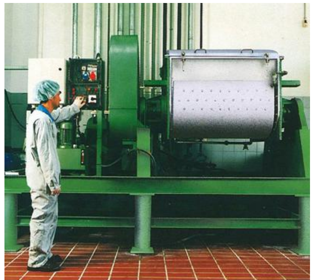
PSG Industrial Sigma Mixer with Jacket
